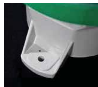
Installation Supports installation on structure using 3 x M6 bolts on a 150 mm diameter.
